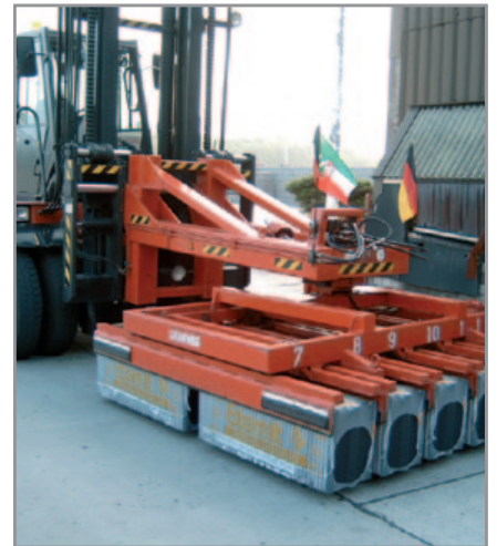
Roof tile clamp DZ6-240 on fork-lift truck
