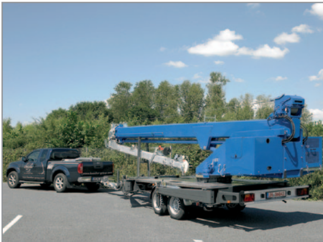
Transport with suitable passenger car due to low dead weight
