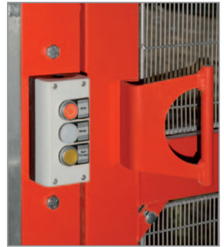
Landing control unit in weather-proof design
